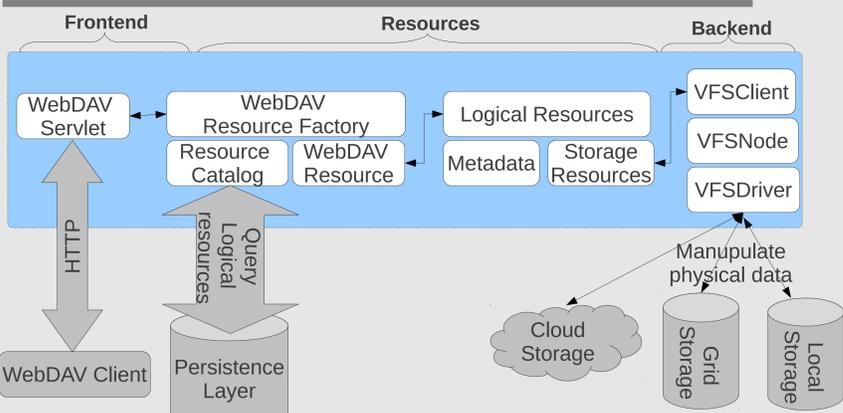
Fig. 3. The frontend layer is a WebDAV servlet. The resources layer is a mapping between the logical resources and the physical data kept in the backend storage. The backend layer is responsible for accessing physical data
