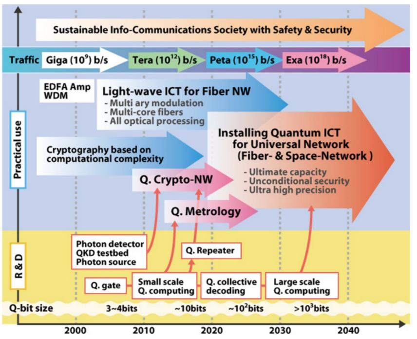
Optical communications are utilizing full potential of the wave nature of light by controlling amplitude and phase for every available modes. This kind of light-wave ICT continues to sustain the increasing capacity demand for future network over a few decades, realizing the network traffic of Peta (1015) b/s.
