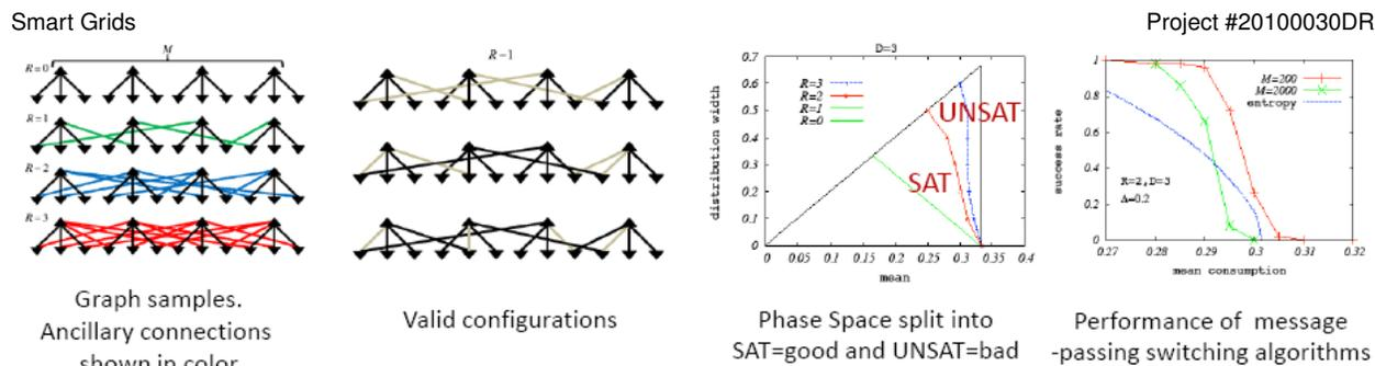
Figure 6: Optimal switching to balance local overload globally without shedding [7].  $M$  is the number of generators.  $R$  is the redundancy parameter. On (c) lines separate the upper right UNSAT corner in the phase space from the lower left SAT corner. The probability of avoiding load shedding is unity in the SAT domain and it is strictly less than unity in the UNSAT domain. (d) illustrates efficiency of the message passing control algorithm.
