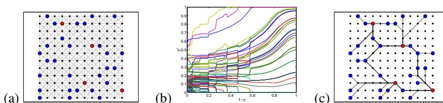
Figure 2: (a) The grid  $G$  showing allowed lines (between nearby grid points), locations of generators (red nodes) and loads (blue nodes). (b) Plot of optimized conductivities  $\bar{y}$  as the control parameter  $1 - \gamma$  is varied from 0 to 1. (c) The sparse solution for  $\gamma = .01$ .
