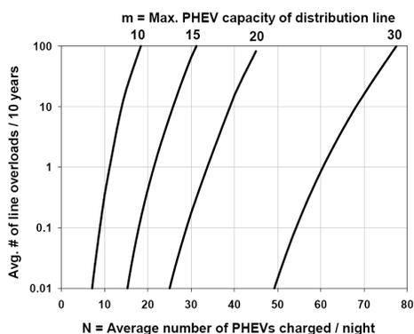
Figure 5: Overload probability for a M/M/m queuing model of PHEV charging, where  $m = 10, 15, 20, 30$ .
