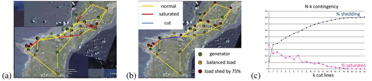
Figure 7: Sample of the Guam transmission grid, consisting of 103 buses (of which 23 are generator buses) and 116 lines. (a) shows a sample original configuration, (b) shows  $N - 1$  contingency (one line cut) for the original sample with maximum amount of load shed, (c) plots the percent of load shedding and the percent of the number of saturated lines at each value of  $k$  for  $N - k$  contingency.
