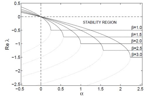
Figure 8: Stability map for a quasi-static model of power grid from [15].
