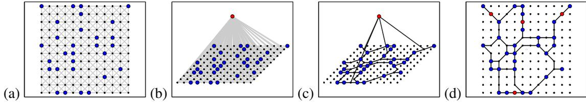
Figure 3: (a) Grid  $G$  showing allowed lines (between nearby grid points) and locations of loads (blue nodes). (b) Extended network including “master generator” connected to all possible generator sites. (c) Sparse network obtained by optimization procedure. (d) Corresponding optimized placement of generators (red nodes).
