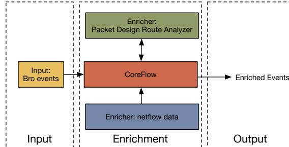
Figure 1: CoreFlow correlates input data from Bro to NetFlow and uses the enriched data to query the route analyzer. Finally, it outputs the security event with additional data from both enrichers.
