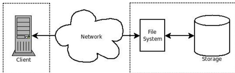
Figure 1: Network Attached Storage
