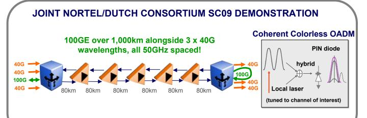
40G and 100G traveling over mixed fibers with NO fixed dispersion compensation!
